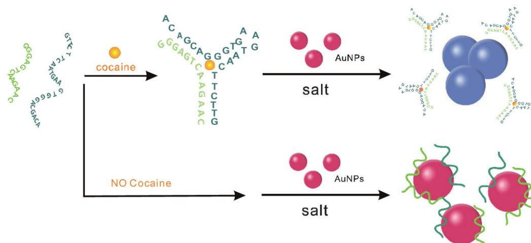
**Scheme 1.** Scheme for the engineered cocaine aptamer and the visual detection of cocaine based on the red-to-blue color change of gold nanoparticles.
