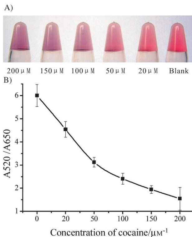
**Figure 2.** Visual detection (A) and the titration curve (B) for cocaine assays with a 10  $\mu\text{M}$  aptamer probe. The y axis of the titration curve stands for the ratio of UV/Vis absorption at 520 nm and 650 nm.
